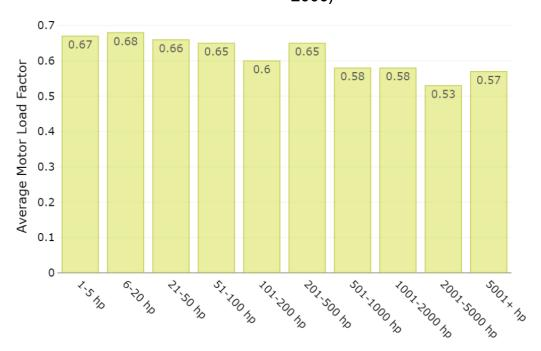
Figure 11: USA Motor average load factor – industry (Rao, 2021)
