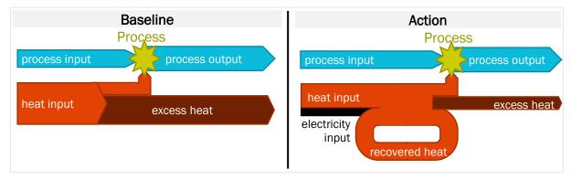
Figure 3: Schematic illustration of feedback of excess heat into the process
