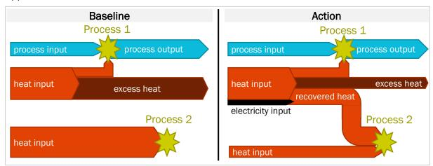
Figure 4: Schematic illustration of on-site use of excess heat for other applications
