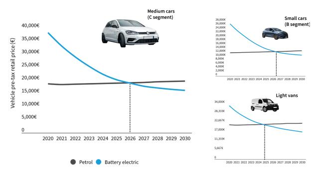
Figure 8: Evolution of costs for different segments of petrol and electric vehicles in Europe
